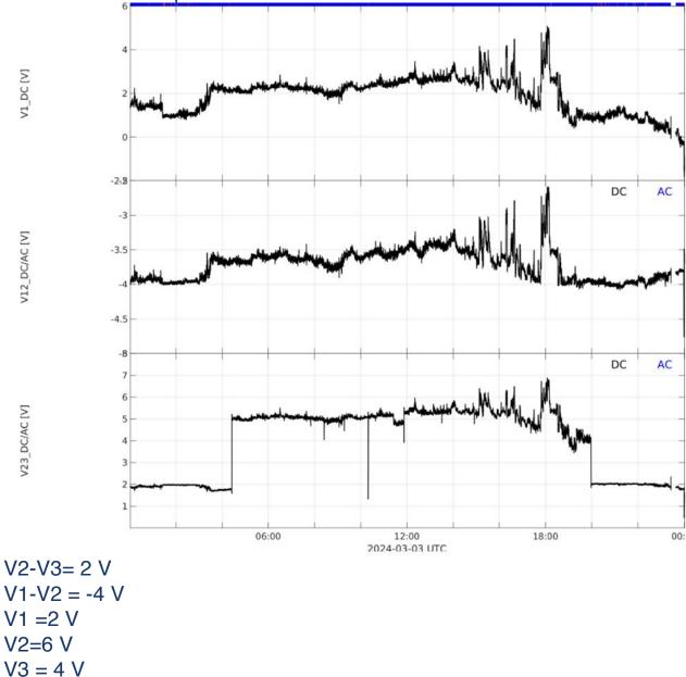
According to LFR F3 measurement during the anomaly we can determine the DC potential in Antenna 3:
