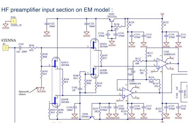
Due to this unexpected latchs up the input section was simplied, but some transistors remains:
