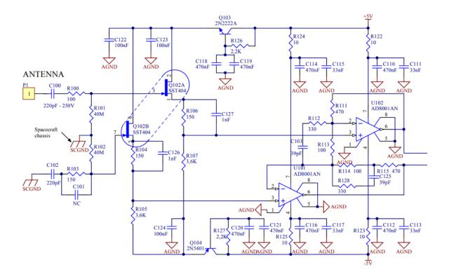
With this modification, on ground, the input transistors never latch-up again.
