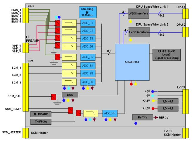
Figure 3: LFR block diagram
