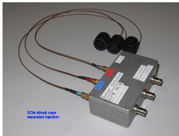
Figure 9. SCM injection setup
