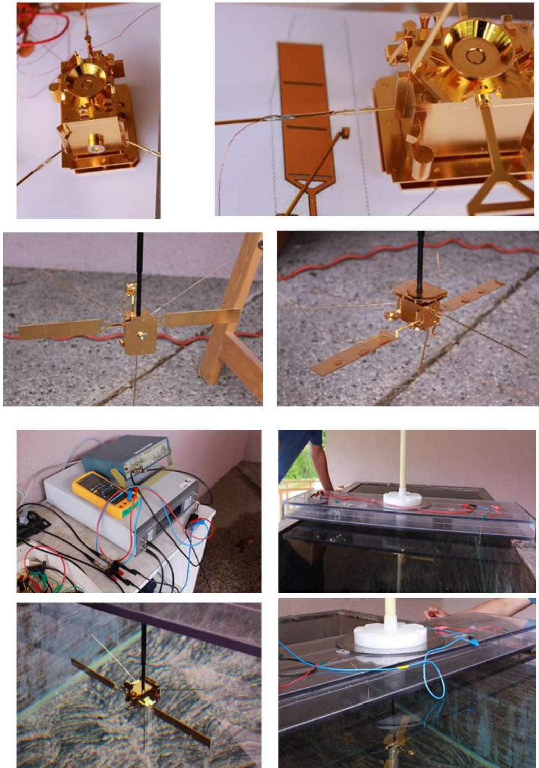
Figure 16. Rheometry measurements of the RPW antennas in a water tank. The top panels show the gold plated Solar Orbiter model.
