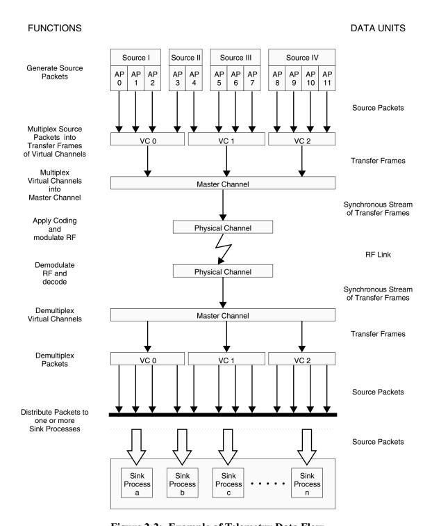
Figure 2-2: Example of Telemetry Data Flow
