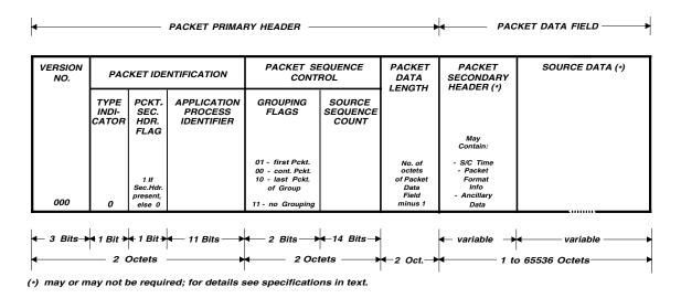
Figure 3-3: Source Packet Format
