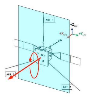
Measure of AKR having a pure circular polarization (V = +1 or -1) to properly estimate the antenna gain, effective length and vector direction.
