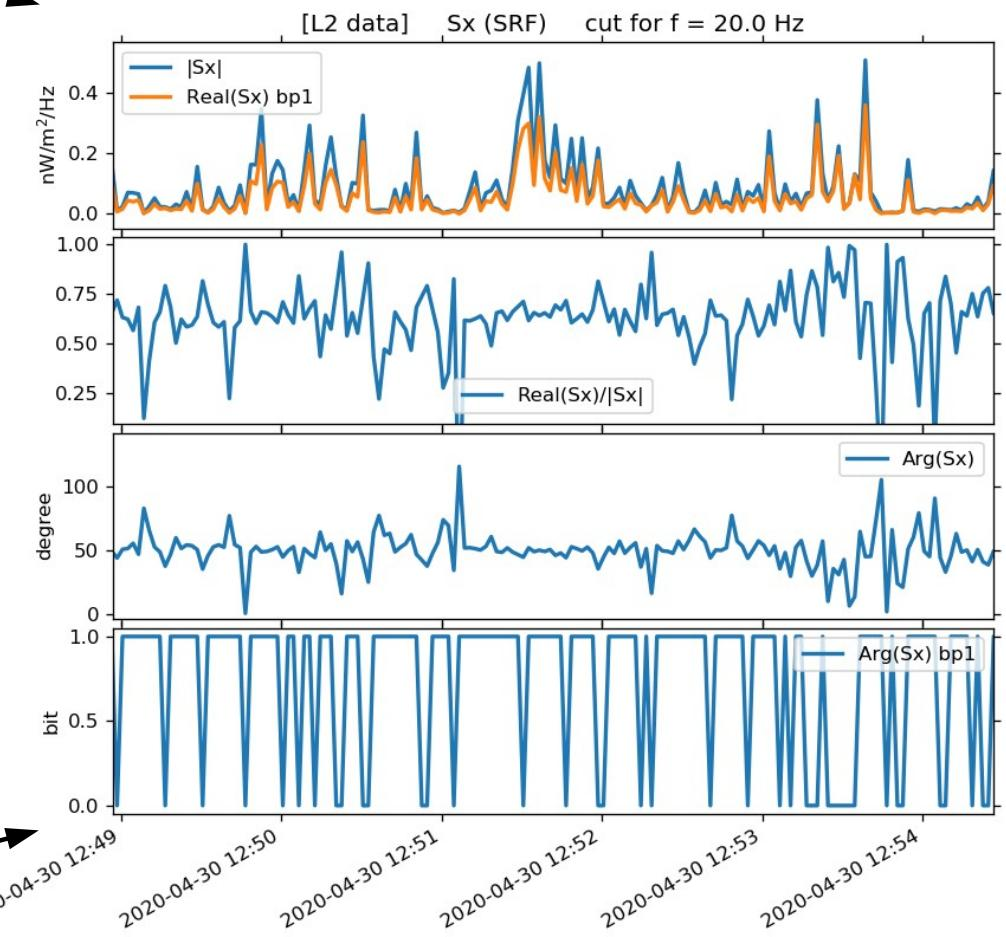
Parallel propagating whistler waves are expected to have a **purely real** Poynting vector (there is no longitudinal component which could contribute to an imaginary part)
